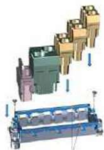
装配前松开滑动边框 Loosen sliding border before assembly
